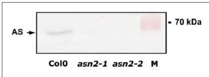
Fig.2 Absence of ASN2 protein in leaf extracts of asn2-1 and asn2-2 mutants.
